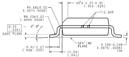
CONTROLLING DIMENSION IS MILLIMETER
