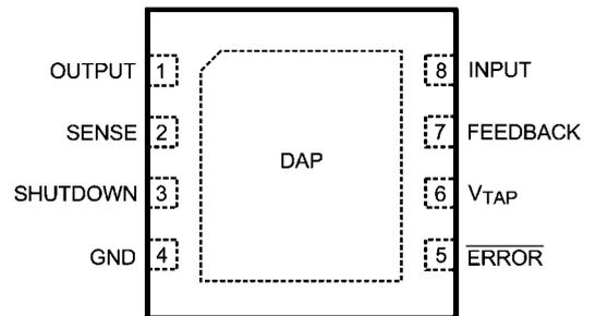
Connect DAP to GND at device pin 4.
